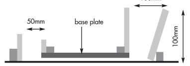
Cross-section of typical grouting formwork
