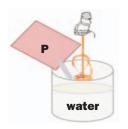
The specified water quantity should be measured in an accurately graduated vessel and added to the mixer. The bagged powder is then
