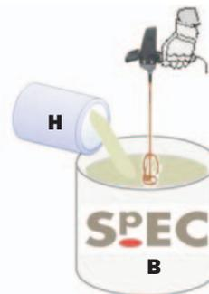
Both of the components should be briefly stirred to ensure that any settlement products are fully suspended. Empty the entire contents of the curing agent into the base component. To ensure that all material is extracted, the insides of the tins should be scraped. The curing agent and the base component should be mixed with a slow speed, heavy duty electric drill and a spiral mixing paddle for at least five minutes and until the material appears uniform in colour and consistency.
