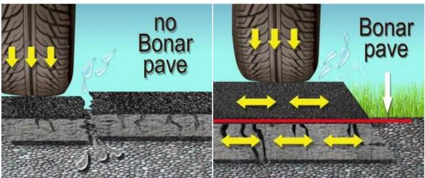
"A high-quality needle punched nonwoven geotextile that, when installed on a bituminous tack coat, performs as a stress absorbing membrane interlayer (SAMI) and inhibits the upward propagation of cracks from the underlying pavement into the overlay". This condition is often referred to as reflective crack control.
