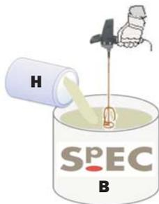
Whilst the internal surfaces of the mixer are still wet with solvent, empty the complete aggregate bag from the **SpECTop EU** pack into the mixer. The aggregates
