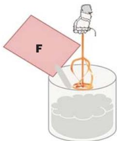
Empty the entire contents of the resin hardener component into the can containing the resin base component and mix until homogeneous. When mixed, the resin
