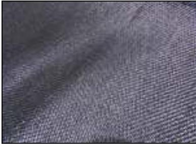
These are high tenacity UV-stabilized polypropylene slit film/fibrillated tape. They have a superior combination of mechanical and hydraulic properties and are suitable for applications involving one or more of the following functions - separation, reinforcement and stabilization
