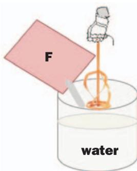
**SpECgrout C1** must be mixed using a slow speed electric drill fitted with a **SpEC Mixing Paddle**. This method is suitable for small quantities and for larger quantities it may be necessary to consider the
