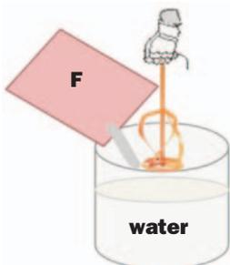
For mixing of single bags, it is acceptable to use a 25 litre steel pail as a mixing vessel, and mixing carried out using a slow speed electric drill (350/600rpm) fitted with
